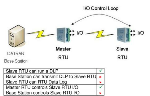
The first part of the configuration for setting up a polled slave is the same in this example as it was in example 1. First, add the Slave RTU module as an IPB expansion module. Second, set up the serial port you will be using to use the "Slave Radio" *Device Type*.
