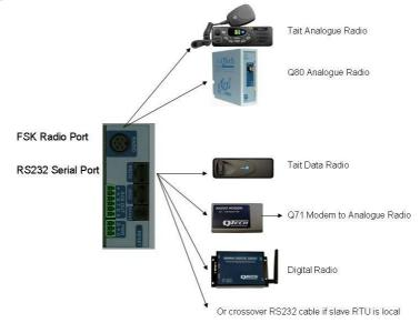
There are many communication options from the Master RTU to the Slave RTU:
