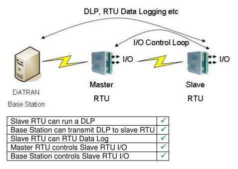
As with the other two examples, the Master RTU must first have its slaves added into the IPB configuration table, and the appropriate serial port should be configured. Again, this example is based on the Slave Radio being a Tait TM81xx data radio.
